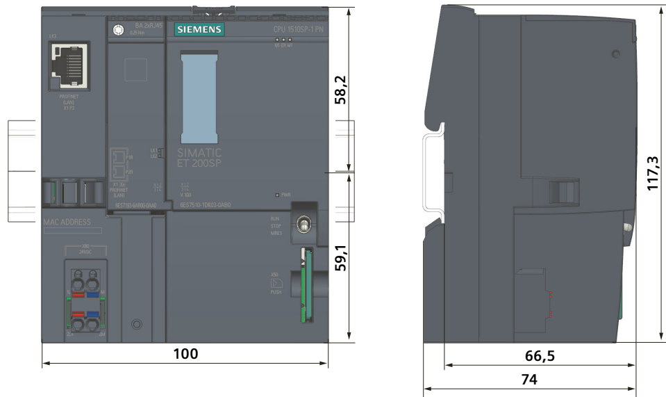
Figure A-1 Dimensional drawing CPU 1510SP-1 PN
