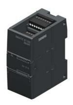
SIMATIC S7-200 SMART, Digital I/O SM DT16, 8DI/8DO, 8 DI 24 V DC, Sink/Source, 8 DO, Transistor 0.75A
