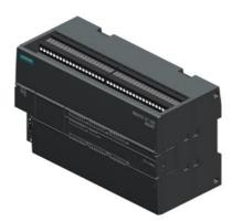
SIMATIC S7-200 SMART, CPU CR60, compact CPU, AC/DC/relay, onboard I/O: 36 DI 24 V DC; 24 DO relay 2A; Power supply: AC 85-264 V AC at 47-63 Hz, Program/data memory 20 KB
